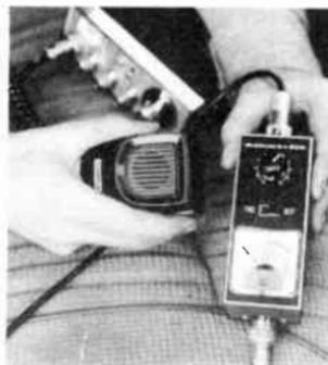
With Squelch open and the car engine running, you'll probably hear a lot of popping noise. In cars with high-energy ignition systems, this interference can really disturb communications.
