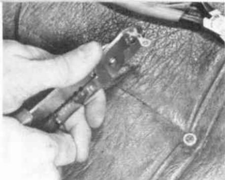
Here's how to crimp a lug onto a wire. Trim the insulation back, exposing about 1/4 inch of bare wire. Twist the strands together. Poke the wire into the barrel of the lug or quick-disconnect terminal. Set the lug barrel into the crimper and squeeze the handles of the tool. The result is a solderless and very solid connection. Lugs are ideal for any wire connection you have to make.
