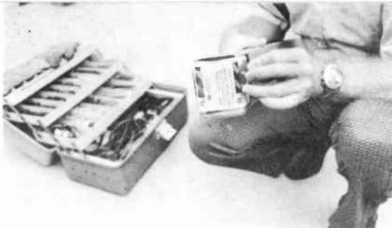
Assemble everything you need before you start construction. Ladder, tool box, coaxial cable, connectors (if your cable doesn't have them attached), pipe for an antenna mast, and of course the antenna parts.
