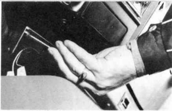
We chose a Cobra model 21 for our sample installation. Its size, in this instance, allowed us to mount it right over the center console in this 1975 Cutlass. Principles are the same for other CB radios and other cars.
