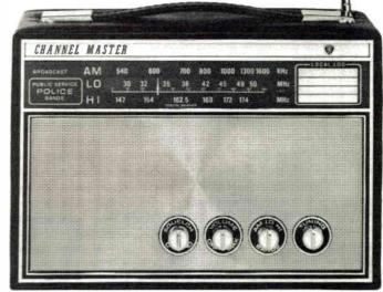
CHANNEL MASTER 6252A is a tunable 3-band receiver that covers both the High Band (147-174 MHz) and the Low Band (30-50 MHz) Police/Public Service frequencies, plus the standard AM Broadcast band. Features variable squelch control, BUILT-IN IIOvac power supply and telescoping antenna. For portable use, it uses 6 "C" batteries. Handsome leatherette case. With earphone & 5' auto antenna connecting cable. 9"w, 7"h, 4"d.......\$ 49.95
