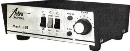
ASTRO ELECTRONICS MACH 100 10/11 Meter 50 Watt Linear has a single grounded-grid 6LQ6 final tube. AM/SSB switch. Transistorized keying requires only ½ watt of excitation. Ideal size for mobile use! DC model comes with Transistorized Power Supply and heavy duty mobile mounting brackets. Approximate dimensions: 3"h, 8"w, 9"d 6 pounds (Illegal for use on 11 Meters in USA.)
