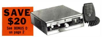
JOHNSON MESSENGER 320 is a 12vdc, 23-channel CB transceiver. Combination S-meter/RF output meter allows visual monitoring of received and transmitted signals. Meter and Channel Selector are illuminated. Built-in noise limiter. Paging feature. External speaker jack. Supplied with crystals for ALL 23 channels, microphone, and mobile mounting bracket................................\$199.95
