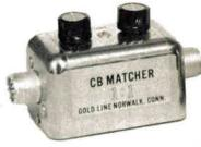
GOLD LINE GLC-1046 Antenna Matching Network stops power loss due to high SWR. A perfect SWR is I to I If your SWR is 1.5 to 1 you're losing up to 20% of your transmitting power. If your SWR is 2.1 you're losing 30% of your power. Simply insert the GLC-1046 Antenna Matching Network between the transmitter and the antenna lead-in with a SWR meter and tune for minimum SWR . . . . . . \$9.98
