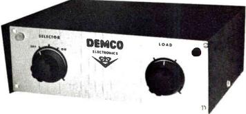
DEMCO "Demon" Base 50 Amplifier for 10 & 11 Meters provides 50 watts of power output with 31/2 watts drive. Uses two 6JE6C's for maximum plate dissipation and reliability. Utilizes low-pass input filter. Simplified controlled loading - one adjustment. 9-3/8" wide x 3-3/5" high x 9-1/4" deep. (Illegal for use on 11 Meters in USA)......\$99.95
