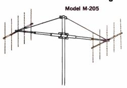
A Kit designed for easy installation of any pair of 3, 4 or 5 element beams or quads. Designed for effective wind loads of 100 mph. Special telescopic seamless aluminum alloy tubes. Extend to optimum spacing of any properly designed pair of beams or quads. Complete phased hook up harness and clamps provided for all models except Boss 303 and 304. The Boss 303 and 404 require additional phasing harness, part No. 15D113 at \$12.92.
