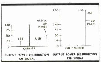
A normal AM signal is composed of three basic segments: a carrier, an upper sideband, and a lower sideband. The carrier conveys no information and serves no useful purpose but consumes a great deal of the five legal watts of power and produces the "silence" that tells you a station is on the air even when no one is talking. All of the intelligence is conveyed in the two sidebands, but these sidebands are mirror images of each other.
