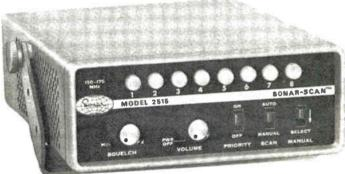
The SONAR AUTO-SCANNER is an FM monitor receiver that will signal-search and automatically lock a signal on any of 8 programmed channels. A Priority Channel signal will lock to the exclusion of all other signals. Carrier Delay allows you to hear mobile callbacks (if on the same channel). Manual selection is accomplished by Slow-Scan technique. I17vac or 12vdc. 7" x 2½" x 8½" Sonar Model FR-2514 for 25-50 MHz FM. \$189.95
