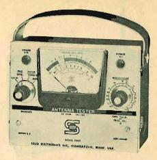
Like most antenna testers, SECO's unit is completely self-contained and self-powered.
