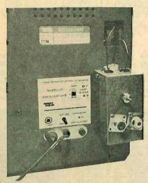
The oscilloscope, because it indicates peaks, is the best CB modulation meter the CBer can use. Unfortunately, the low-voltage output from a CB rig hardly gives a usable pattern. But add our outboard CB Modaptor to your scope and even a 1-wattoutput will fill a 5-inch scope.
