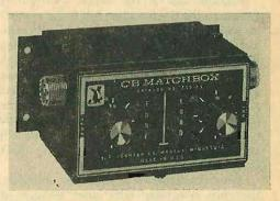
Johnson Matchbox matches rig and antenna.
