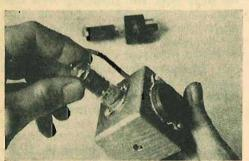
Tester is simplicity itself to use: simply plug Tester into outlet, tube into Tester.
