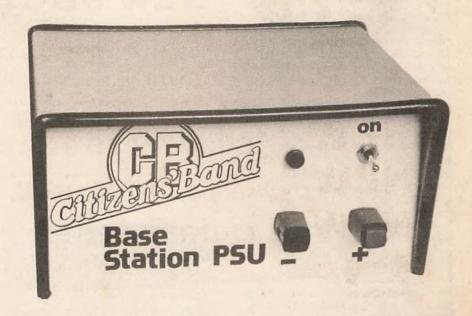
The supply, and anything connected to it, is protected from overload (like an accidental short circuit). If the current drawn exceeds 3.5 amps the output voltage and current 'fold back', the voltage dropping rapidly, and the current output is then less than that available at the full 13.5 volts.
