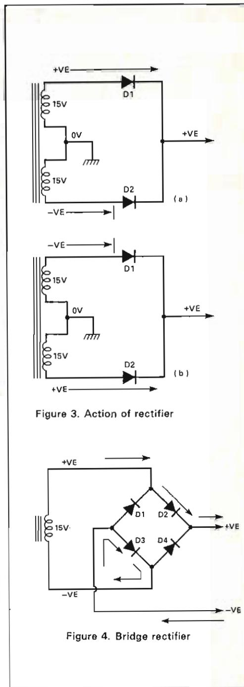
Figure 3. Action of rectifier
