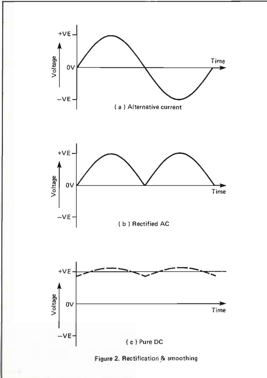
emerging. When the top end of the winding is positive and the bottom negative as shown the current flows through D2 and D3 which are forward-biased. D1 and D4 are reverse-biased in this condition. During the next half-cycle when the positive and negative from the transformer are reversed, the current flows through D1 and D4, and
