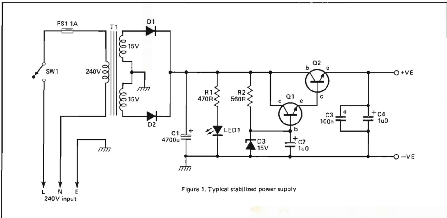
Figure 1. Typical stabilized power supply
