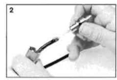
Slide coupling ring over the connector. Strip back the PVC and screw the connector body onto the cable.
