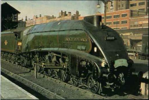
Perhaps the most famous class of steam engines, the streamlined A4 pacifics which ran all the major LNER express trains before and after the war. Designed for high-speed, light trains, (Mallard, preserved at the NRM, York, holds the record speed for steam, 126 m.p.h.). During the war they handled trains of up to 850 tons between Kings Cross and Newcastle. Several examples are preserved in working order, including this one, the Union of South Africa.
