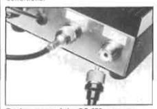
Replacement of the SO-239 antenna connector at the rear of the set will not be allowed, except by the manufacturer.
