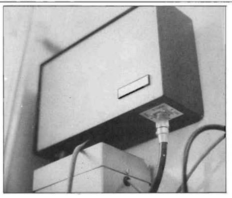
The transmitter (note the 50 ohm output and use of thick low loss type cosx).
