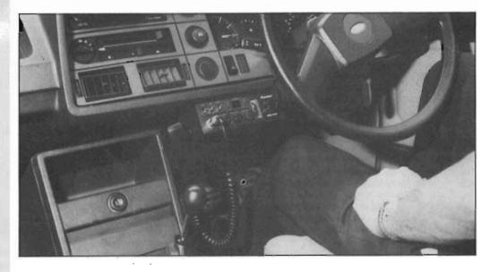
PRESIDENT AR 44 40 channel AM Mobile Radio. Controls: Powerl volume. Squelch. Mike gain. RF Gain. Switches: ANL/ OFF. PA-CB. CH9-OFF. BRITE-DIM. Features: "S"/ RF meter. Digital channel indicator. Automatic Modulation Control.
