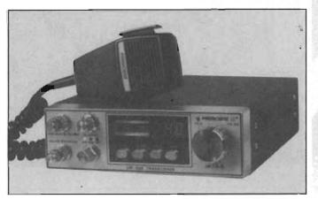
PRESIDENT AR 14-4 40 channel AM/ SSB Mobile Radio. Controls: Power/ Volume. Squelch. Mike Gain. RF Gain. Clarifier, Switches: NB/ ANL-OFF. PA-CB, CH.9-OFF. BRITE-DIM. Mode. Features: "S"/ RF Meter. Digital channel indicator. TX/ RX Mode + CH. 9 Indicators. Automatic Modulation
