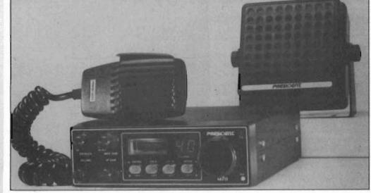
FIVENINER (shown in-dash) 40 channel AM Mobile Radio. Controls: Power/Volume. Squelch. RF Gain. Switches: PA-CB. Delta.
