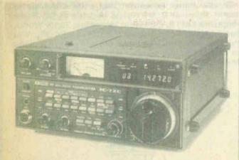
This HF transceiver has a memory which can be recalled, even when on a different band to the one in use and covers from 100kHz to 30MHz. Its cost is justified by such features as an automatic antenna tuner unit, provision for AM, SSB, CW (Morse) and RTTY and needs no tuning or loading. The Icom 720 costs £883.
