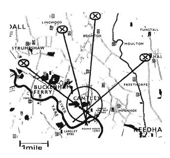
Fig. 4. Initial testing of a DF loop antenna with the ald of a fixed station at a known position. See text.
