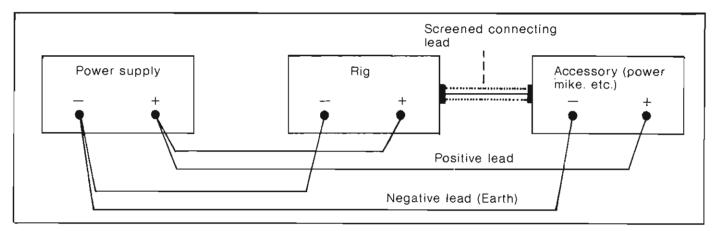
Fig. 1. Showing normal method of connecting on occessory.
