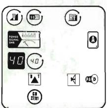
includes controls for volume, squelch, RF gain, Delta tune and channel select. Switches are provided for power, attenuator, SWR and calibra-
