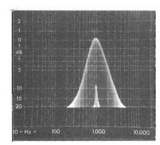
Flg. 3. Audio frequency response (typical) transmit through to receive. Ref.: 1,000Hz - Odb.
