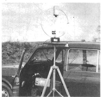
The CB radio 27MHz DF loop set up on a stand and with a compass attached. Photo taken during test trials hence the reason for the special field strength meter that can be seen.
