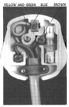
The correct way to wire up a 13-amp plug. Notice how all the wires are trimmed to the correct length except the Earth, which has been looped and that there is no bare wire showing. The cable clamp has been tightened over the outer core and the correct-volue fuse has been fitted.
