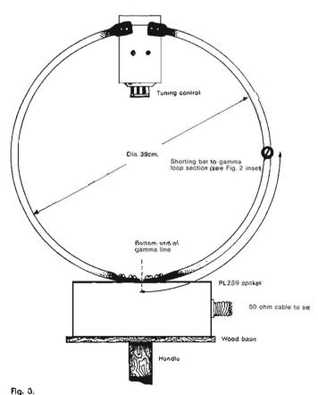
figure for the showing how the assembled loop can be mounted on a platform with handle attached.
