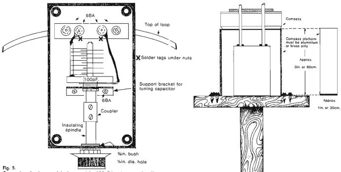
Connections for the top of the loop and the 100pFd tuning capacitor. Note the extension spindle on the capacitor to prevent hand capacity effect when tuning the loop.
