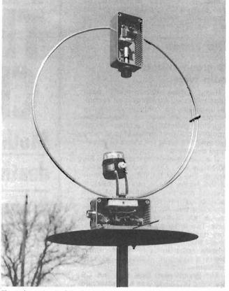
Photo shows detail of the finished loop antenna with upper and lower box lids removed. Note small potentiometer visible in lower box is not used (see text).
