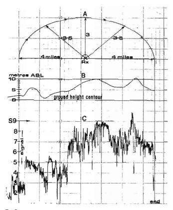
Fig. 5. (A) Elliptical test course with Rx or point of reception. (B) Ground height contour over course. (C) Signal variation over course (pen chart).
