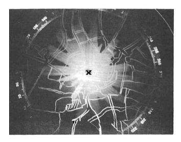
Fig. 4. How radiation from an omni-directional antenna can be affected in a built-up town area (see text). Transmitting station at X'.
