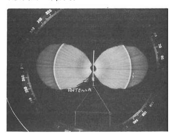
Fig. 2. Perfectly symmetrical vertical angle radiation from a vertical halfwave antenna in clear surroundings.
