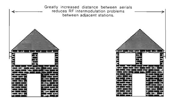
Sketch (not to scale) showing how the position of aerials can bring about an improvement in the RF intermodulation problem.
