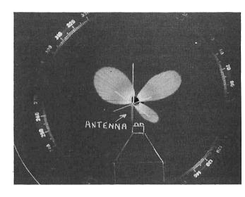
Fig. 6. Radiation pattern (vertical angle) of an omni-directional groundplane antenna constructed to the Home Office specification with a baseloaded radiating section 1.5 metres long. Radiation is at an angle too high to be of any real use. The small lower lobe is due to radiation from the ground plane.
