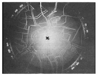
Fig. 5. Assuming no effect whatsoever from buildings as in Fig. 4, radiation from a vertical antenna would be exactly equal in all directions around it. Hence the term amni-directional.
