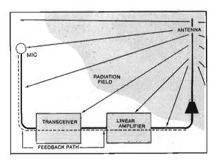
Fig. 2: The radiation field in the immediate vicinity of an antenna is very intense. The radiation can be picked up by the microphone (and through connecting leads etc.) and cause instability, high VSWR and severe interference to other services e.g. TV, broadcast radio and hi-fi systems etc.
