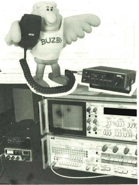
Demonstrating, with the aid of a spectrum analyser, that the rigs work on the legal frequencies.
