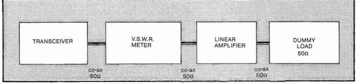
Fig.1: Checking the self VSWR of a linear amplifer
