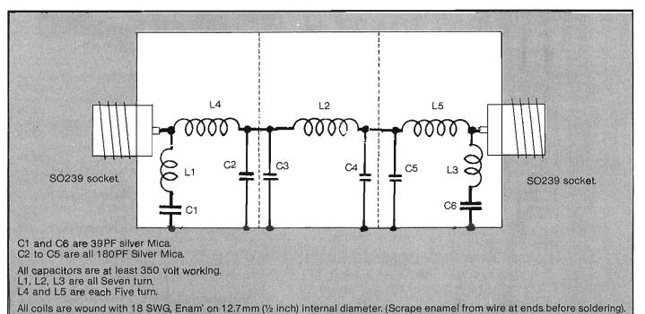
Screens are soldered along both sides and bottom edges.
