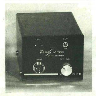
By removing power wasting peaks from the speech waveform and unwanted frequencies the average 'talk power' can be increased by up to THIRTY TWO times.
