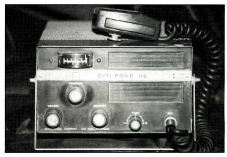
An older CB radio uses relays to switch from transmit to receiver.
