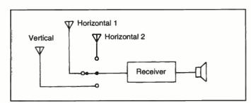
Fig. 3. Three antennas and one receiver (or CB transceiver) typ- Fig. 4. Adding second receiver to installation brings better allify cost-cutting hookup. Switch selects antenna.
