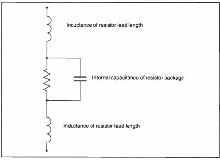
Figure 1- A resistor used at high frequencies may look like this in a circuit!
