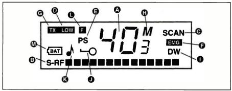
Display panel features are: A. channel indicator; B. signal/RF meter; C. scan; D. low power; E. PS (power saver); F. emergency channel; G. TX (transmit); H. "M" indicates preset memory; I. DW (dual watch); J. key lock; K. beep; L. function mode; M. "BAT" (low battery indicator).
