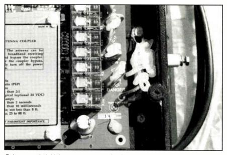
Relays to switch high antenna currents in big radios are required over PIN diodes.
