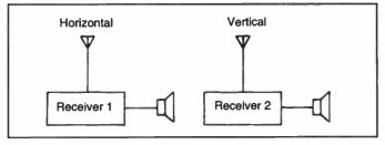
Fig. 1. Simplest setup uses two receivers and two antennasone horizontal and one vertical.
