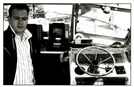
A CB radio (next to the steering wheel) on a boat also needs noise elimination procedures.
