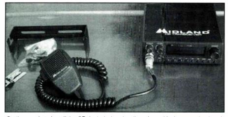
Getting ready to install the CB; included and well-packaged is the mounting bracket, mic bracket and hardware and power cord. (Photo by Harold Ort)
