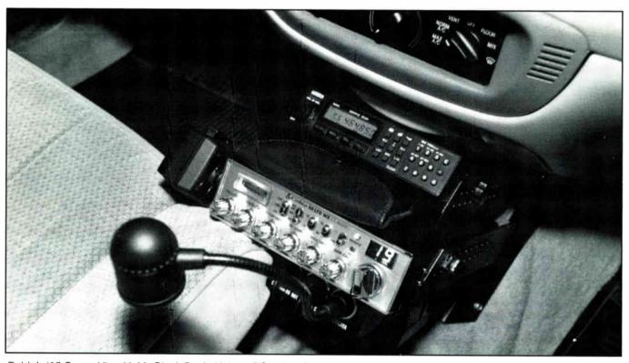
Robin's '95 Crown Vic with his Black Rack, Uniden BC 760 XLT 100 channel scanner, Cobra 29LTD WX Classic CB, Cadet Dash Light, Radio Shack extension speaker, and Gall's three-hole outlet box, You can't see it, but Robin uses an Austin "Spectra" scanner antenna and Larsen NMO 27 low band CB antenna. (Photo by Robin W. Hartford)
