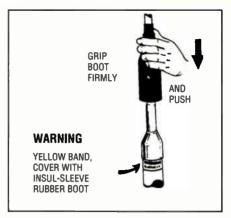
Getting "the boot" to slide down the fiberglass antenna requires a couple of minutes and some patience. Otherwise, the antenna is as easy as 1-2-3 to set up. (Courtesy Shakespeare Electronics, Inc.)
