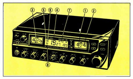
The layout of controls on the 2010's front panel is impressive. At number "7" notice the frequency display. This drawing, taken from the instruction manual, is typical of the detail throughout the instructions. (Courtesy Cobra Electronics Corp.)
