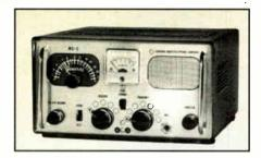
General Radiotelephone's MC-5 was a popular early multi-channel transceiver with a tunable receiver and large S-meter.
