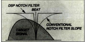
with a big carrier on AM, a DSP filter can notch out the annoying tone. Filters with two notch capabilities offer twin tone annihilation.
