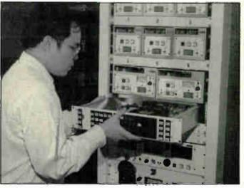
A National Weather Service technician assembles a new generation of weather radio transmitters which will give the NWS offices new capabilities for broadcasting severe weather watches and warnings to very specific geographic areas, so listeners in other areas won't be bothered by warnings that don't apply to them. (NOAA Photo)
