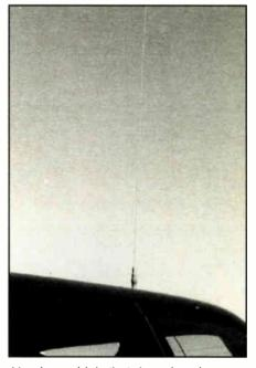
Here's a vehicle that doesn't make many trips through the bank's drive-up window. That's a 102" whip on the roof. Remember, the longer antenna is better. (Photo by Kent Britain)
