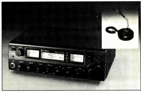
The Cobra 2010 GTL WX is a full-featured AM/SSB CB. Here's the 2010, also showing the professional-looking and feeling Cobra desk microphone. The instruction manual includes wiring instructions for users interested in using a different mic with the 2010. (Courtesy Cobra Electronics Corp.)
