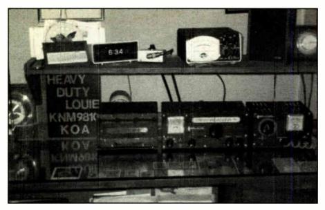
How about these Buddy modular units? In the center is a Buddy RC-11B tunable receiver. At the right, there's a Buddy TX-11B, which operated on six channels. These were sold primarily in southern California during the early years of Class D.
