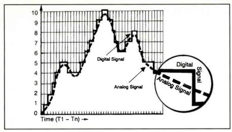
The digital signal is rounded off to the closest step voltage each time the analog signal is sampled, called DSP "quantization." (Courtesy Craig Clark, KR6T)
