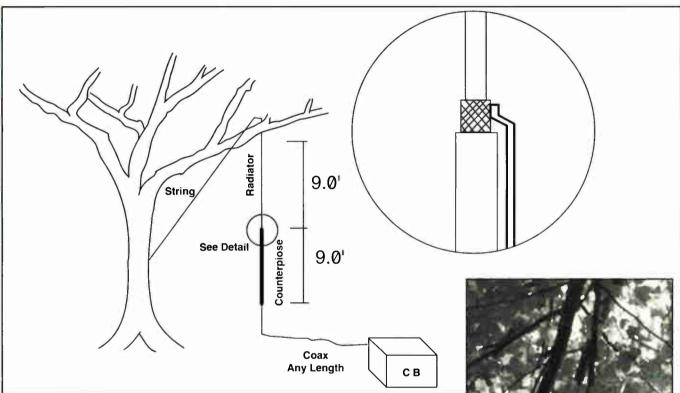
The homemade Backpacker CB antenna. For a few bucks and a little time, this can be your emergency antenna.
