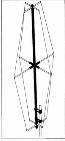
Don't want to use a rotor? Consider an antenna like the Signal Engineering Company's Thunder 8XB. It's nearly 15 feet high and includes a coax switch to change directions. It weighs about 11 pounds. (Photo courtesy Signal Engineering Company)
