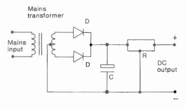
Fig. 5. Basic circuit of regulated power supply (see text).
