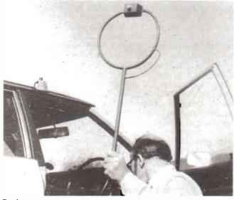
Fig. 6. The UFO CB radio direction finding loop antenna by Whitehorse Communications. This employs a gamma matching system and is fully tunable for the 27MHz band. It is only 10in. (approx. 26cm.) in diameter and is supplied with co-axial connecting cable and plug.
