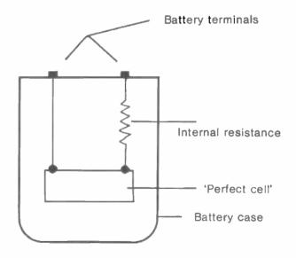
Fig. 3. Although not a 'real' resistance, the internal resistance of a cell can be treated as a separate item wired in series with a 'perfect cell'.
