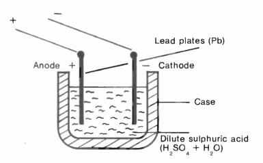
Fig. 1. Bosic cell construction.
