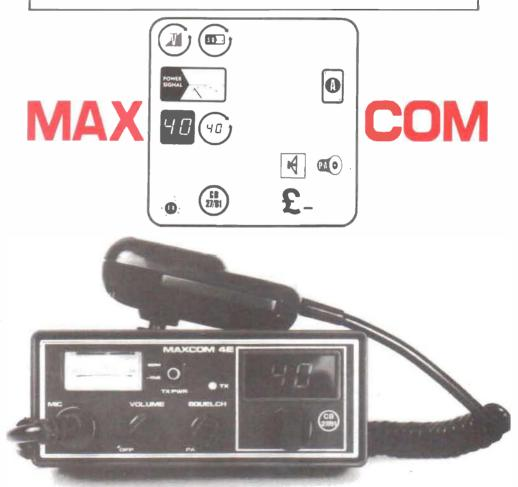
costed the parts used to build the set and it came to approximately £60.00 at retail value. We don't know how they do it but keep it up! It is about time that more sets had the attenuator switch on the front panel which makes it far more easy to use. The only two complaints with the set are the moulded din plug which has to be cut off when a fault occurs and the fact that the public address facility cannot be left permanently connected as most breakers that use this facility prefer to do.
