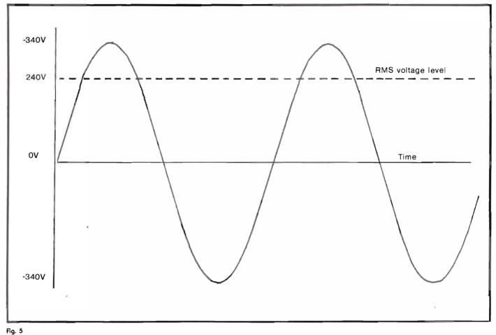
The real voltage from the AC mains, compared to the RMS voltage
