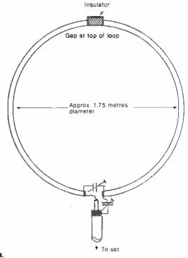
Fig. 4. Although very accurate, a loop with a circumference of a half-wavelength is far too large for operation on 27MHz when this has to be carried out quickly from different positions, perhaps as much as three or four miles opart, i.e., the size makes it too cumbersome for partable operation.
