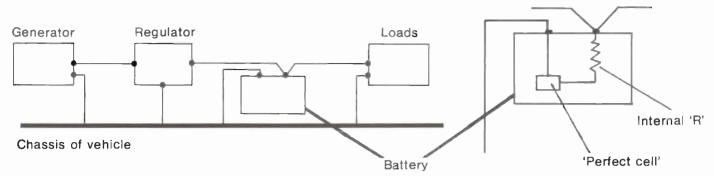
Fig. 4. Showing how the internal resistance of a cell cames *between* the actual battery and the external circuits. In an extreme case ('R' open circuit) the battery would not have ony influence in controlling the final voltage. A good battery would have a very low internal 'R' and would stabilise the voltage. Dirty terminals, etc., can have the same effect as a high internal 'R'.
