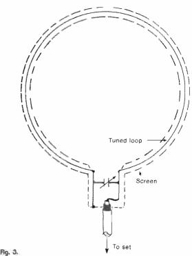
The screened loop has a very accurate response and does not suffer from antenna effect as explained in the text, such loops are, however, very difficult to construct and the matching and tuning circuitry is much more complex than the basic arrangement shown.
