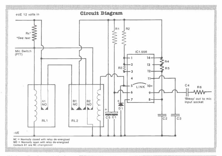
400 ohms coils resistance at 12 volts. If problems are encountered with the unit 'chattering' or failing to switch properly this will be because RL2 has too low a resistance capacitor for the particular rig. To overcome this, C1 can be increased in value. The whole unit is built into a small plastic box with a mic socket and a short lead with a mic plug on it.
