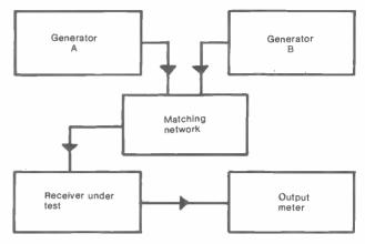
Generator A and the receiver are tuned to the same channel
