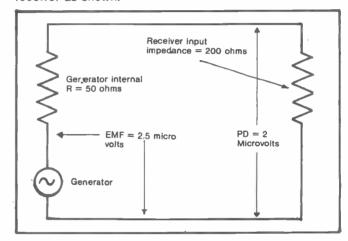
Fig. 2 When the receiver impedance is not matched to the source the output EMF is no longer split in equal amounts between the two. This would of first sight seem to imply that this receiver was the more sensitive as the actual EMF required is less. However, it in fact requires four times as much power for the same result as the receiver in Fig. 1.
