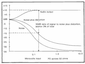
Fig. 4 Typical graph showing how the audio signal recovered from the modulation, harmonic distortion and noise vary with microvolts input. It shows that full limiting is reached at around 0.1 microvolt. 39dB signal to noise plus distortion is reached at around 0.2 microvolts. 20dB quieting is reached at around 0.1 microvolt. It also shows that the best signal to noise that can be expected from this particular receiver is about 40dB with inputs above 10 microvolts.
