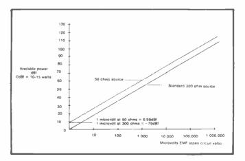
Fig. 5 Graph showing relationship between EMF and available power in dBf into the 300 ohm standard impedance, with the 50 ohm impedance shown for comparison. Note that for a given EMF the power into 50 ohms is 7.78dB (six times) more than for 300 ohms. This shows the importance of correct matching between aerials and receivers, etc.
