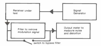
The signal generator is set to produce a fully deviated signal with a modulating frequency of 1KHz. The filter is adjusted to remove the 1KHz signal from the output, leaving only the noise and distortion to be read by the
