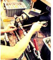
Archer antennas are hand-crafted for quality. This expert is putting the final touches on loading coils.
