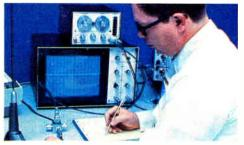
A spectrum analyzer is used to check new and experimental antenna designs.
