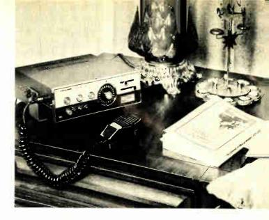
A mobile sideband rig costs less than a base station. By adding a 110 volt power supply, a mobile rig can become an instant base station, and you can still toss it into the mobile unit.
