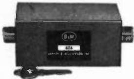
A B&W low pass filter will end interference with your neighbors TV reception. B&W Model 424 is a three-section low pass filter which installs in the antenna coaxial line. Reduces all frequencies within the TV band by 60 db (a reduction of 1-million times).
