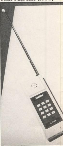
readiness for a call which it will signal by bleeping, and talk is self explanatory. The pushbutton dial is similar to existing Post Office pushbutton phones, and operates faster than existing exchange equipment, which means that the dialling clicks on the line go on long after you've finished pressing buttons. Once the call is connected you can swan about the house, the garden, wherever, anywhere that isn't more than about half a mile away, in fact.
