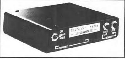
CB 206 scans through all 40 (AM/FM) CB channels, automatically locking on to any active channel.
