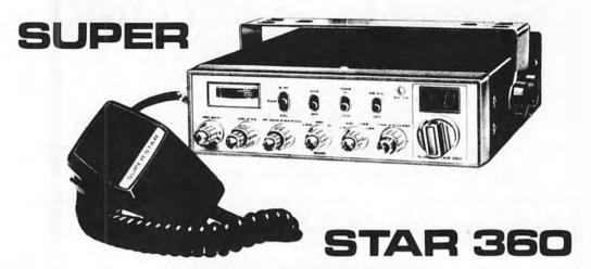
General Specifications: Channels 120 AM, 120 USB, 120 LSB and 120 CW. The Frequency Range is 26.965 to 28.940 MHz, with Frequency Tolerance at 0.005% and Frequency Stability of 0.001%. Overall Cabinet dimensions are 203mm W. x 64mm H. x 235mm D. The meter is illuminated and indicates relative RF power output and SWR on Transmit, received signal strength.
