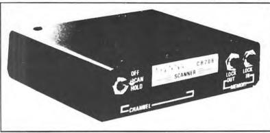
CB 206 scans through all 40 (AM/FM) CB channels, automatically locking on to any active channel.
