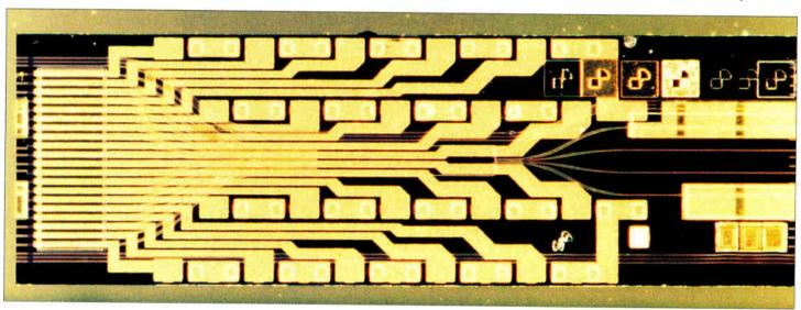
8-Wavelength Laser Array. (Photo courtesy of Belicore.)
