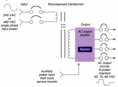
down the coax to the RF amplifiers, fiber nodes, network interface units and telephony equipment, SNET selected conventional 60-and 90-volt, 60-Hz, quasi square-wave power.
