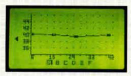
When equipped with the Multiplexer Option, the 9580SST accepts signals from up to 8 separate test points and analyzes sweep & ingress from each individually, returning data to as many as 6 SSR field units (A thru F) connected to it. Announcing the Trilithic 9580 Sweep and Ingress Monitoring System
