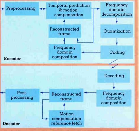
one frame to another. This is known as "interframe" coding. Sending information only about the changes dramatically reduces the amount of data that has to be transmitted. In the MPEG process, bidirectional prediction is used to help forecast motion. This step buffers several frames so that the preceding and succeeding images can be examined and compared to determine how much motion takes place and where the moving objects should be placed.
