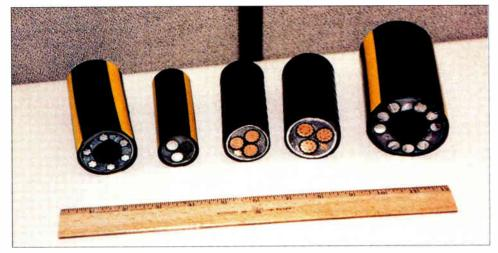
View of the various cable types used in the construction of the overall system. From the left, the cables are: six conductor branch cable with innerduct used for side branches, two conductor branch composite cable used for single node branches, 2/0 copper CLX used in underground ducts, 4/0 copper CLX used in underground ducts and nine conductor feeder cable used in primary aerial backbone.
