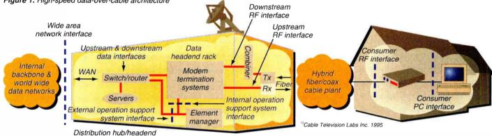
Figure 1: High-speed data-over-cable architecture
