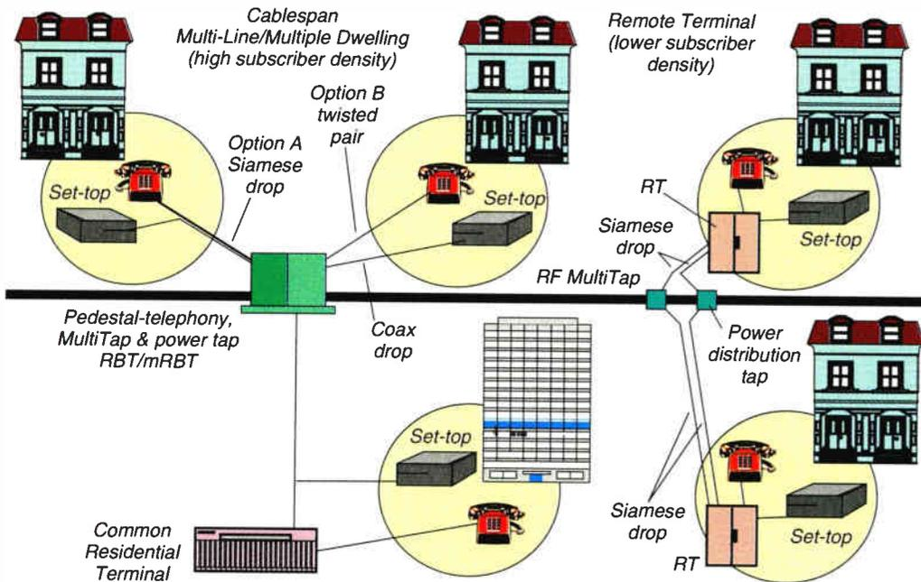
nesses, or a Remote Subscriber Terminal (RST) for multiple dwelling unit/business applications. In the RSU upstream, TDMA is used on a 1.6-1.7 MHz carrier to handle 30 DS-0s. The RST uses TDM in both the upstream and the downstream paths.
