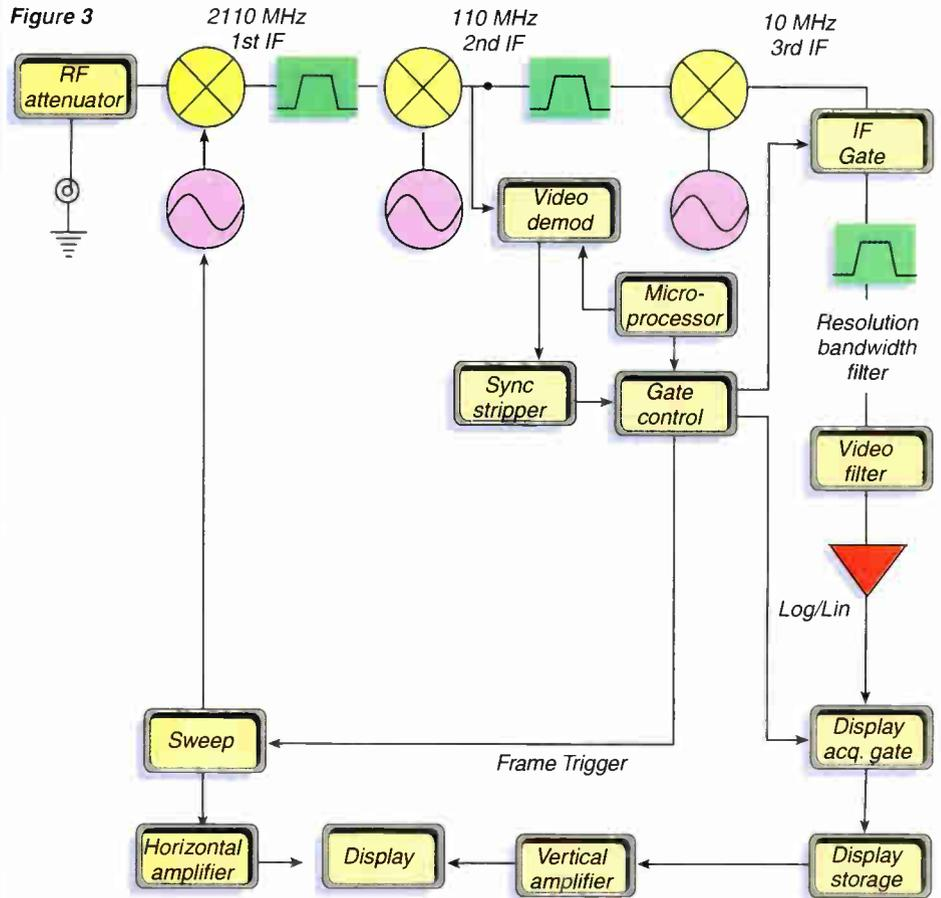
Signal path for gated measurements.
