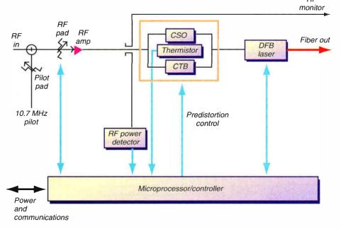
Figure 3: DFB transmitter block diagram. The laser is predistorted for both second and third order distortions.
