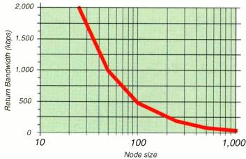
Figure 2: Return path bandwidth vs. node size
