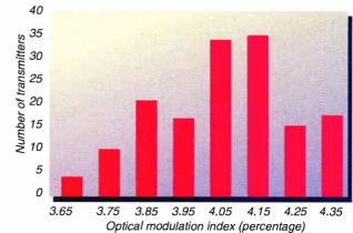
Figure 4: Optical power and modulation index histograms for 150 transmitters. Mean optical power is 12 mW (10.8 dBm), and mean modulation index is four percent per channel.
