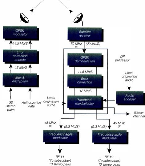
Figure 1: Basic DP transmission link
