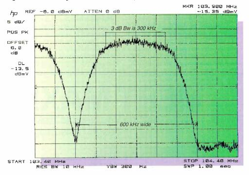
Figure 4: One discrete digital cable radio channel occupies 600 kHz of bandwidth
