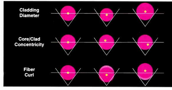
alignment for connectors and mechanical splices.
