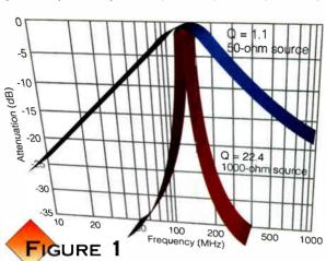
same effect can be obtained by keeping RP constant and varying  $X_P$ . Thus, for a given source and load resistance, the optimum Q of a resonant circuit is obtained when the inductor is a small value (low value of inductance) and the capacitor is a large value (high inductance). Therefore, in either case,  $X_P$  is decreased.
