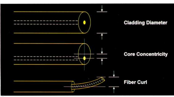
One answer is improved fiber geometry characteristics and the advanced splicing technologies they make possible. Together, tight geometry tolerances and more efficient splicing techniques can provide better results at lower costs.
