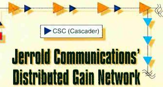
Designed as a method of maintaining existing trunk/bridger locations in overspaced situations. The concept reduces or eliminates the need to upgrade cable and the time needed to upgrade the system. The topology is compatible with CAN and FBB.
