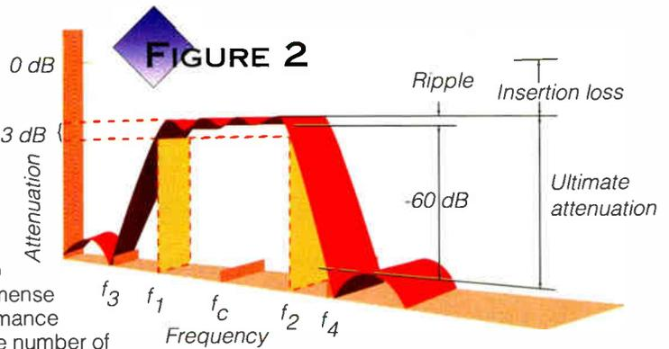
the difference between the upper and lower frequency ( $f_2-f_1$ ) of the circuit at which its amplitude response is 3 dB below the passband response. For this reason, it is often called the half-power bandwidth.
