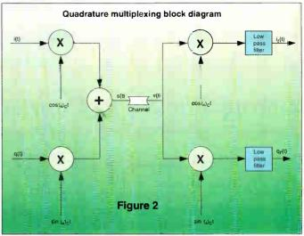
This shows that both I and Q control the amplitude and phase of the QAM signal and the signal can be completely described at any time t by its amplitude and phase. In the 4-level data case this leads to the signaling states shown in Table 1.
