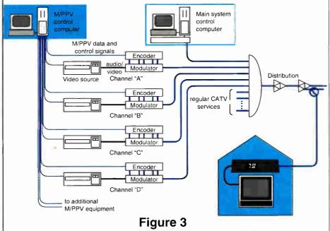
nels will be needed to multiplex this title. Therefore, four channels of spectrum space would be needed, as well as four individual program sources—usually tape machines or laser disc players.
