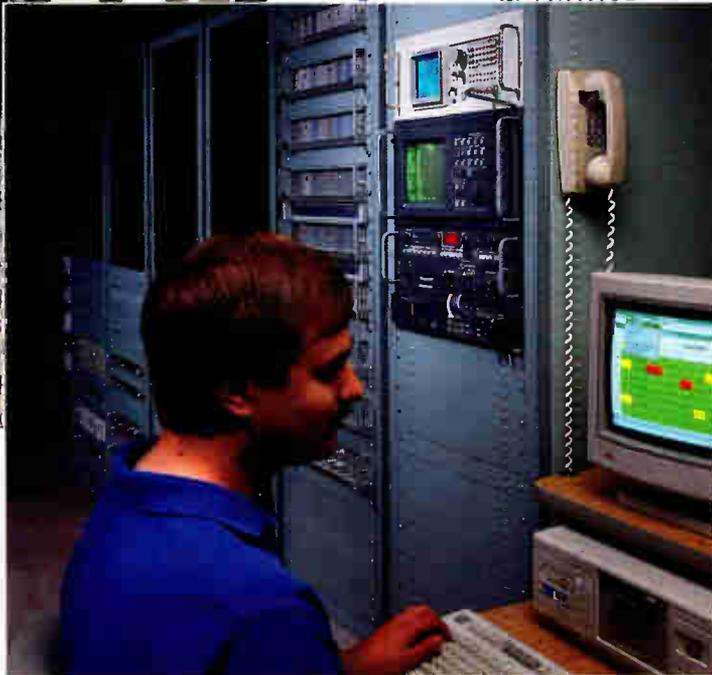
(ABOVE) THE CMP500 CABLE TELEVISION MEASUREMENT PACKAGE — COMPLETE BASEBAND VIDEO AND RF MEASUREMENT CAPABILITY, INCLUDING ALL FCC PROOF-OF-PERFORMANCE REQUIREMENTS.
