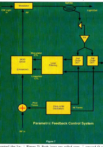
loop may be used to control the linearizer bias condition.
