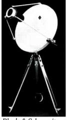
New from Rhode and Schwarz is the model AC 008 portable broadband microwave antenna, covering a 1 GHz to 18 GHz frequency range. The antenna is particularly useful for detecting RF signals and field for
