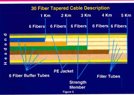
splice location. The remaining express tubes in the cable continue to the next splice points, leaving fibers within these express tubes undisturbed. Filler tubes replace the buffer tubes after fiber taper points, thus maintaining the uniform outside diameter of the cable (see Figure 5).
