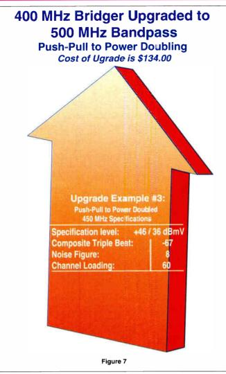
noise input and power doubler output, had a measured improvement of 13 dB CTB and a noise figure that became better by 3 dB.
