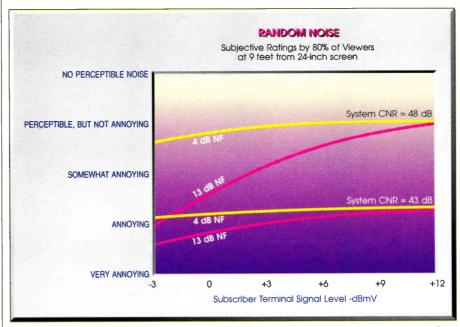
proposed "minimum" standards are simply a "means of defining an acceptable quality of service at the worst subscriber location and thus a better quality of service to the average subscriber." However, even 48 dB system CNR is significantly degraded by the 13 dB NF.
