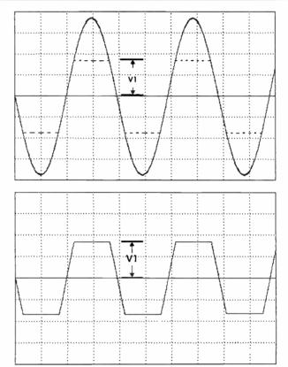
ILLUSTRATION OF I'R LOSSES IN ZENER TYPE CLAMPING CIRCUIT
