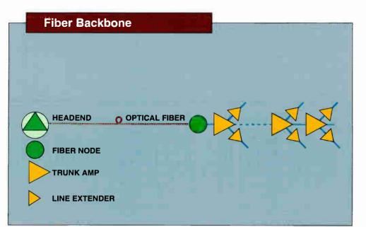
Conventional fiber backbone reduces active cascades as compared with coaxial trunk system. This improves picture quality and service reliability while extending system range. Sumitomo full bandwidth transmission and plug-in filters provide flexible split-channel loading. A/B switch provides system redundancy.
