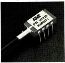
AT&T Microelectronics' 1310 Astrotec® long-wavelength P/N photodetector
