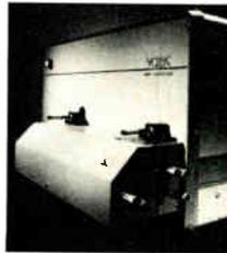
in less than two minutes and offers repeatability (typically 0.003 dB RMS on a short fiber length). The standard wavelength range is 750 nm to 1750 nm and customized units can cover wavelength ranges from 350 nm to 5500 nm. In addition, the S25 now offers mode field diameter measurement across a 750 nm to 1750 nm wavelength range. For more details call, (818) 955-8927.
