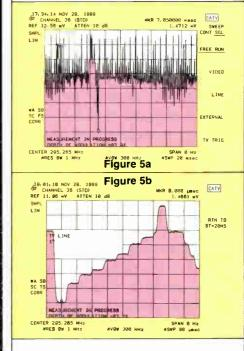
referenced to a 4-MHz noise-power bandwidth, and read out on the display (Figure 4).
