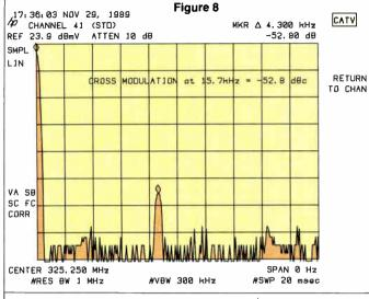
tuning-off from carrier center to measure composite second-order distortion.
