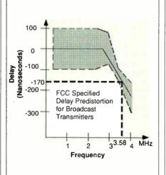
delay near the edges of its passband (read color subcarrier) relative to the center of its passband (read luminance).
