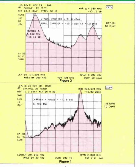
Beats Measure combines several functions to make a single, convenient function for identifying intermodulation products and interference signals.
