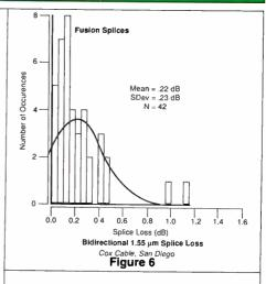
Splicing times were nearly identical for both approaches, although the fusion splicing machine did show sensitivity to ambient temperature and humidity variations. Bidirectionally averaged OTDR splice-loss results, at both 1310 nm and 1550 nm, for this completed installation are shown on Figures 3 through 6.
