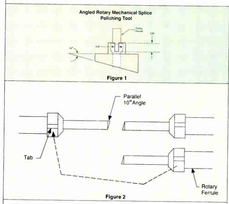
The Angled Rotary Splice (ARS) was designed for cable TV application to yield improved performance over the AT&T Enhanced Rotary Mechanical Splice (ERMS). This article will present data from field applications that illustrate performance characteristics equal to or better than fusion splices.
