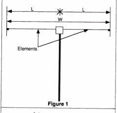
accuracy of the measurement are width and length. Width is derived from the following formula:  $W = 11808 \div F$ .
