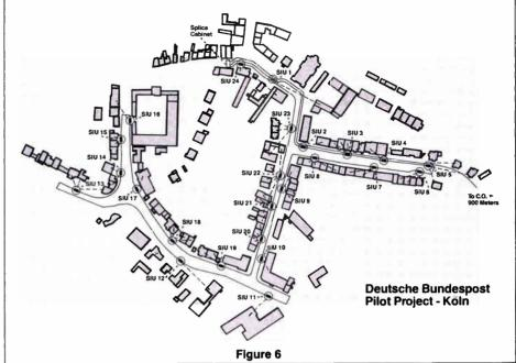
CATV hub is provided with a broadband feed from the local cable system containing 23 video channels plus FM radio service. Service is provided to 96 CATV connection points from the same 24 SIU locations.
