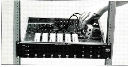
If you've ever had to add or change a channel on your headend in the field, you know how difficult and time consuming it can be. On the other hand, our new *modular* Geomax-10 processing system makes the job a snap. You just plug in a new module. Each of the 10 modulators or processors is a mere 25 cubic inches
