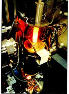
An outside vapor deposition blank is lowered into the draw furnace to begin the fiber drawing process.
