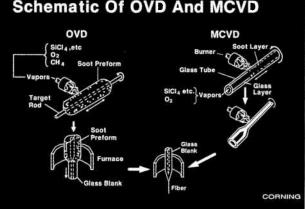
that eventually becomes an integral part of the finished fiber. The most commonly used IVD process is the Modified Chemical Vapor Deposition (MCVD) process. In this method, a glass tube is placed in a lathe and rotated while a burner flame traverses back and forth along the length of the tube to heat it.
