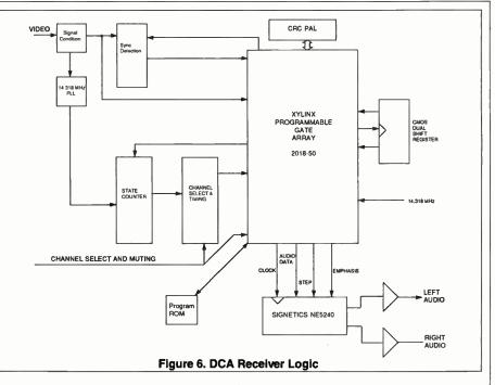
the insertion of externally generated data into the bit stream. Each "line" has provision for the insertion of enough bits to have an aggregate data rate of approximately 420 KB/sec. Some of these bits are reserved for future use and as encryption information channels. This capability for data transmission is not the only means of transmitting data through the digital audio signal. In addition to externallygenerated data to be inserted in each
