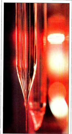
A partially drawn outside vapor deposition blank is displayed to demonstrate how a blank is drawn down to fiber.
