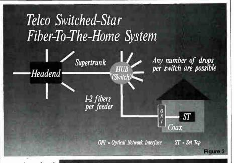
transmits only 40 AM video channels. Only two of those are simultaneously tunable per household. The signal-to-noise ratio at 48 dB is in the same category of today's all-coax systems. By detailing the mechanical requirements of each neighborhood hub, the extensive real estate requirements became clear. The representative noted that a similar system in France passed about 100,000 homes, achieving only a 10 percent subscriber penetration rate.
