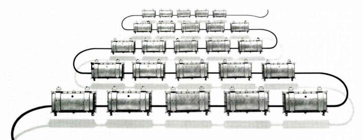
It's well known that line amplifiers directly diminish CATV signal quality. Yet today's cable distribution systems rely upon an architecture in which signals must pass through as many as 60 amplifiers before they reach a subscriber.
