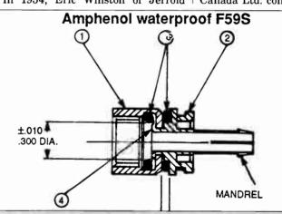
Electronics developed a solderless and easy to install connector called the F59.
