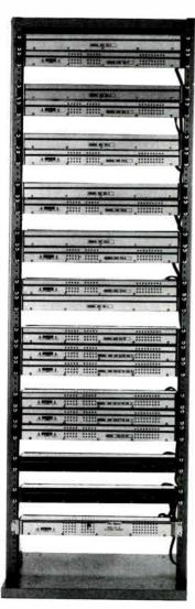
Conventional 10 Channel Off-Air Processors and Modulators
