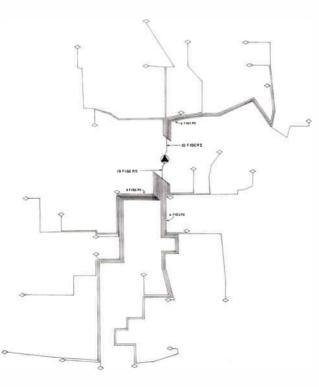
NODE LOCATION AND FIBER ROUTING FOR FOUR IN CASCADE
