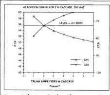
to meet the required performance criteria. The use of three line extenders in cascade requires the addition of up to 147 percent more line extenders than the "quad power" choice, and in that case, 46 percent of the distribution system required the use of three line extenders in cascade.
