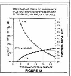
mitted the direct replacement of the amplifier locations, one can see that the "reach" is inadequate to replace the original 28 in cascade, and some sort of hub network will be required to complete the upgrade from 270 to 550 MHz.
