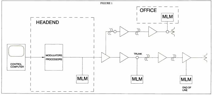
age that can withstand the extreme environmental conditions required to become an integral part of a CATV or LAN distribution system. This product will allow detailed frequency response measurements to be made at multiple points in the system without the expense of sending a truck to each location. System maintenance will be improved and down time reduced. The Magnavox Line Monitor (MLM) is the first product to combine these features
