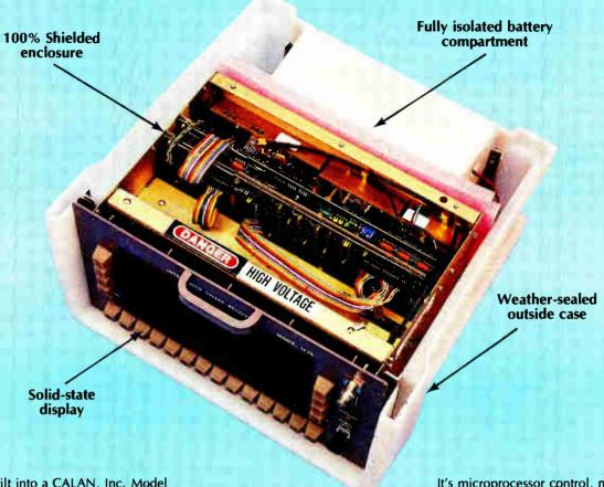
Reliability built into a CALAN, Inc. Model 1776 Sweep Receiver is very apparent from the outside: the totally weather-sealed case; the ruggedized overall construction; the moisture-sealed key covers on the front panel.
