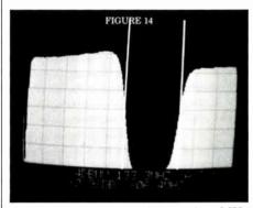
Swept response of notch filter (6.4  $\overline{MHz}$  suck-out).
