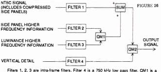
Filters 1, 2, 3 are intra-frame filters. Filter 4 is a 750 kHz low pass filter. QM1 is a quadrature modulator with the subcarrier frequency about 3.1 MHz and all sidebands 'hidden' in the Fukinuki holes. QM2 is a quadrature modulator where the carrier is the normal picture carrier.
