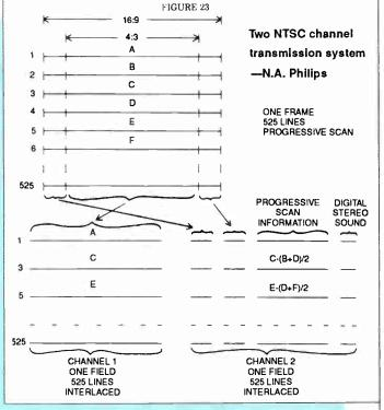
portion of the picture would not appear in current receivers as a result. With a receiver designed to recover this signal, though, the side panels would be stretched to their proper size. This technique results in low bandwidth side panels.
