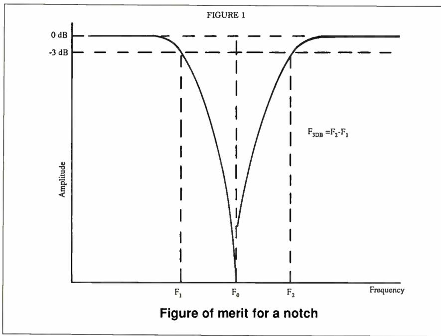
at the subscriber's home. The goal of the design of this filter is to remove the interference without producing perceptible artifacts in the recovered television signal.
