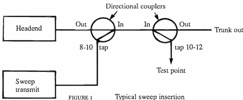
FIGURE 1 Typical sweep insertion
