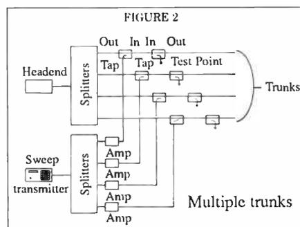
no carriers are present. Sweep response testing provides a means to align and verify the amplifier's performance. It also provides a pictorial of the effect of the cable and other components on the sweep signal over the entire system's bandwidth.
