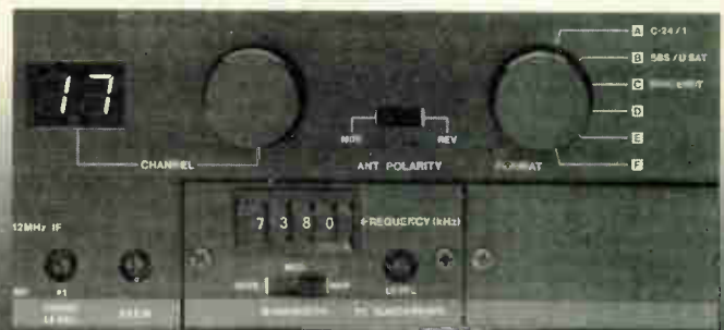
Format control enable selections of desired satellite system. Direct-reading channel selector displays transponder-assigned channel. Second selectable subcarrier and space for optional third subcarrier or descrambler modules.
