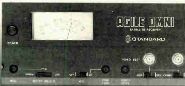
Operating functions including MGC, AGC, AFC, level sets, normal/invert video, clamp/unclamp video, 6-key subcarrier frequency selection, video and IF test points are conveniently located on the front panel. Meter reads C/N ratio, signal strength or center-tune.
