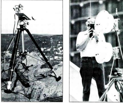
M/A-COM's MA-13CP and MA23-VFM portable microwave transmit/receive units provide flexibility for remote origination and short haul applications
