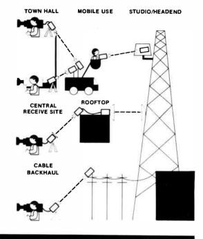
Portable microwave technology isn't just for broadcasters anymore. M/A-COM has devised a Community Access News system for local origination that cable operators can use to their advantage.
