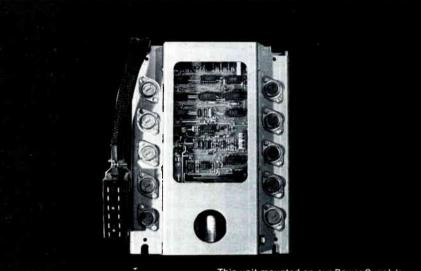
This unit mounted on our Power Supply's door contains the: 1) inverter 2) charging circuit 3) switching
