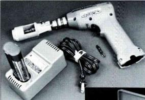
Poleline CorePrep 5 coring and stripping tool
