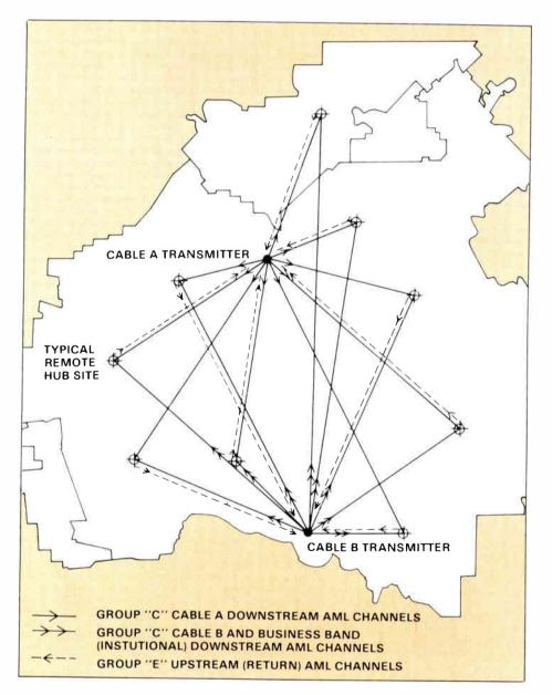
Typical dual cable configuration showing multiple reuse of the CARS spectrum
