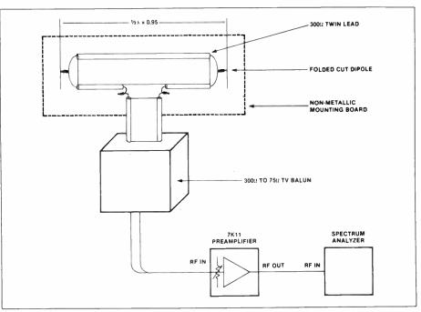
Figure 12-1 Details of homemade antenna and equipment connection for leakage measurements
