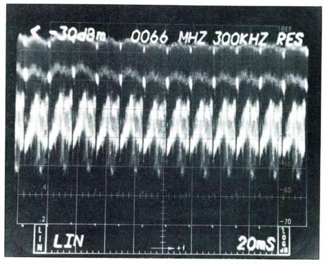
Figure 10-2 Measurement of hum and low frequency disturbance
