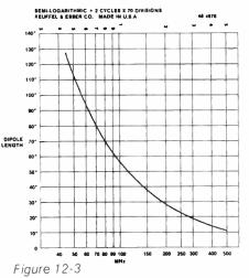
$\supset \lambda$  dipole length vs. frequency
