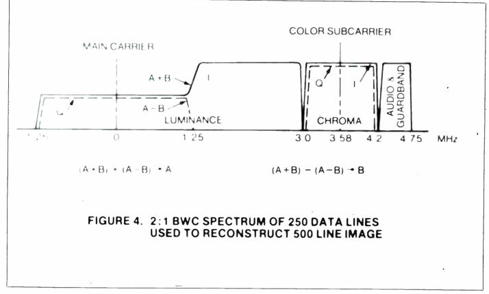
Figure 4 2:1 Bandwidth compressed spectrum of 250 data lines used to reconstruct 500-line image
