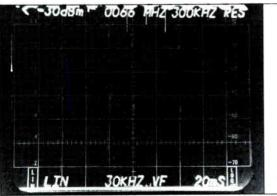
Figure 10-3 Measurement of hum with 7L14
