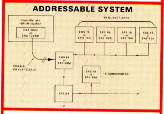
The above system is composed of 3 units a microprocessor control (EAS-1024); a decoder
