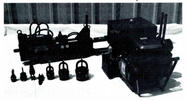
MODEL E4 **Pulls 1" - 4" Pipe** Wt. 199 lbs. Trench Needed — 6" x 6'6" — 2 Men Can Handle Easily Hydraulic Gates Lock Elephant In Trench The "E4" Develops 31,416 lbs. of Pressure at 2,500 PSI.
