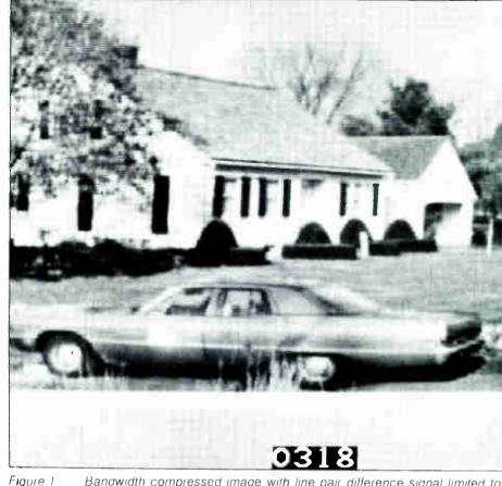
Bandwidth compressed image with line pair difference signal limited to 0.318 MHz bandwidth
