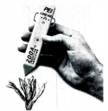
The 200A inductive amplifier is designed to identify and trace wires or cables within a group without damaging the insulation. The probe weighs 2 oz. and has a leather case. A tone from the probe's internal speaker indicates which wire is attached to the tone generating test set. A hand set can be clipped to the ears on either side of the probe if desired.
