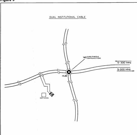
Multiplex Access/Collision Detection (CSMA/CO) philosophy and works on RF frequencies. All stations listen to the circuit. If the link is idle, the station requiring to transmit proceeds and listens for its own signal (echo) to confirm the transmission. Should two stations transmit simultaneously, the transmissions collide and each station attempts to retransmit after a random delay. 20 stations can be handled in a 300 KHz assignment, or 400 in a 6 MHz video channel.
