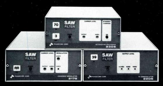
\*SAW... it stands for "Surface Acoustic Wave" Filter. It makes for super reliable vestigial sideband signals with superior performance characteristics. Now it is being delivered in every modulator, demodulator and heterodyne processor that we make, standard or HRC.
