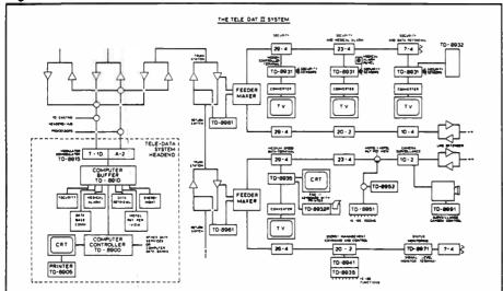
(Regional Interconnect) transmission. Data terminals talking to each other on the same system are coupled by an interlinking of two RS-232C ports. The front end computer is used for system status monitoring and billing records.
