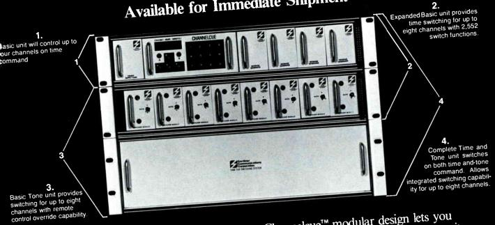
We have finally caught up. For the first time in twelve months, we have units ready to ship. Over a thousand Channelcue<sup>™</sup> systems are now at work efficiently and reliably performing the many video switching tasks in today's increasingly complex cable operations. Channelcue™ modular design lets you buy only what you need. And - yes - it can be adapted for commercial insertion.
