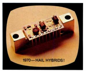
**TRW does it first. Again.** First hybrids for CATV. Elimination of interconnects provides inherent increase in reliability, ease of field repairs. Improved performance over discrete amplifiers.
